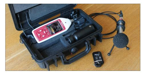
On average, Nick will leave the Trojan in situ for up to 5 days. The Trojan is mains powered with secure cables but it will switch to its own internal batteries if the mains power is lost. When power is restored, the Trojan will automatically restart even if its internal batteries are spent. This allows continuity and Nick knows that they are recording everything over a set period of time.
