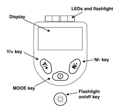
Three panes along the bottom of the display are "mapped" to the keys. These change as menus change, but at all times the left pane corresponds to the [Y/+] key, the center pane corresponds to the [MODE] key, and the right pane corresponds to the [N/-] key. Here are three examples of different menus with the relationships of the keys clearly shown:
